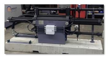
At the conclusion of our 3-year test program, our newly designed coating, **CCI-SS (Seal Saver)**, has produced impressive results. The increased life expectancy of rods coated with CCI-SS is yet to be determined, as none have shown significant
